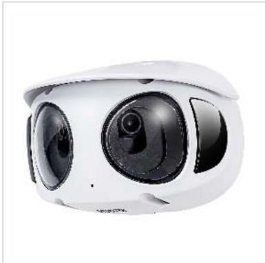
**Outdoor Vandal Dome, 8M 180° Panoramic (4736x 1648), (2x4M sensors), 30fps, H.265/H.264/MJPEG, 2.8mm each lens, D/N, IR 20m, Smart IR III, WDR Pro, PoE, Built-in Mic, MicroSD/SDHC/SDXC, IP66, IK10**
