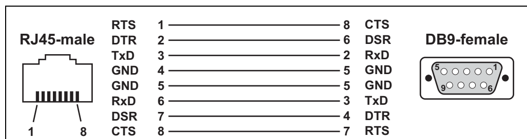
Figure 13: RJ45 to DB9 Serial Console Cable
