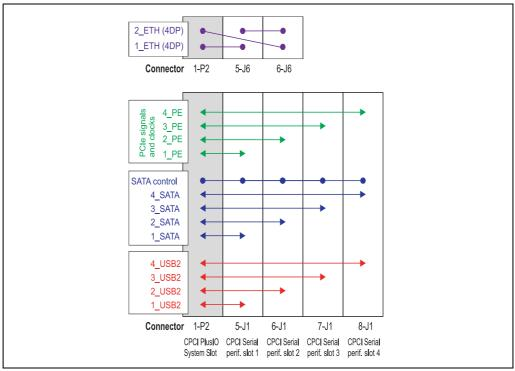
Table 1: Pinout CPCI PlusIO Connector 1-P2 (System Slot)
