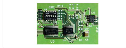
Figure 4: Electronic and mechanical DIP Switch
