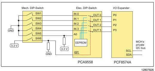
The customer can use either the mechanical or the electronic DIP switch to set the carrier number.
