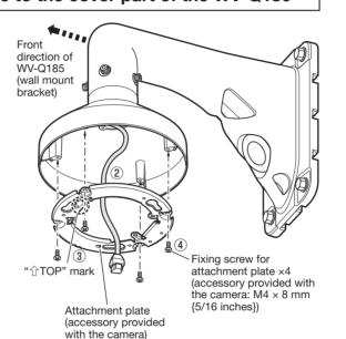
\* The upper right illustration is provided as an example of attaching the attachment plate for a camera model having three attachment mounting screws.
