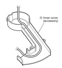
2 Fix (A) inner cover (accessory) using (B) screw (M3: accessory) (Recommended tightening torque: 0.78 N·m {0.58 lbf·ft})
