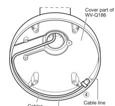
After fixing the WV-Q186 on the WV-Q185, lay the cables as shown in the upper right illustration and confirm that the ends of the cables reach the cable line inside the cover of the WV-Q186.
