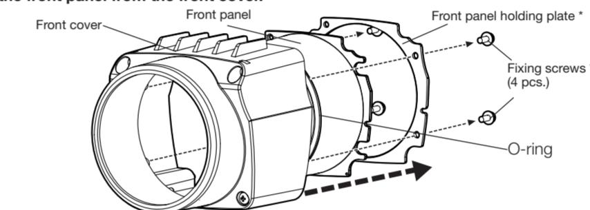
\* Keep the removed the front panel holding plate, and fixing screws (4 pcs.) until using them in Step 3.
