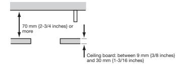
• The thickness of the ceiling board for installation can range between 9 mm {3/8 inches} and 30 mm {1-3/16 inches}.
