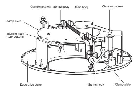
\* Because the triangle mark is engraved on the bracket, it can be seen from both the top and bottom sides.
