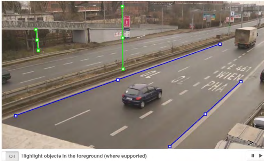
Fig. 73: Draw vertical lines to define the road
