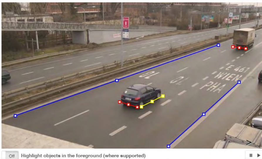
Fig. 78: Draw a reference line (yellow) and give a reference length
