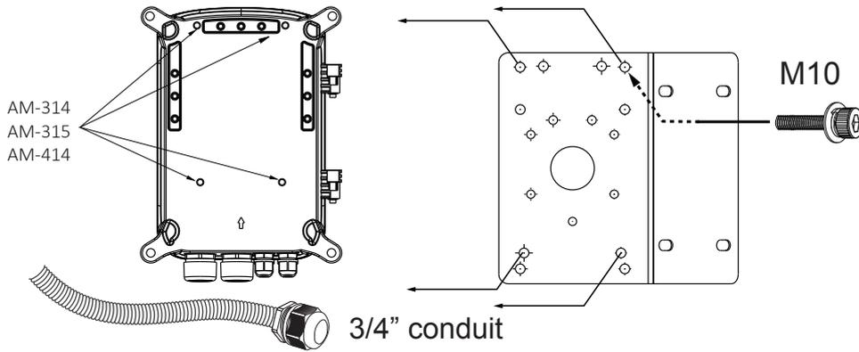
The mounting hole definition is illustrated below. The same mounting hole pattern apply to all pole-mount and corner-mount brackets.
