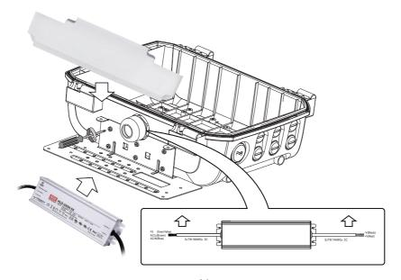
Insatll 3/4" and M16 cable glands and cable conduits to protect the cables and the wiring to the outside of the cabinet. Properly install the cable glands so that the product's IP rating is maintained. If not properly installed, water may seep into the cabinet, causing damage to devices inside.
