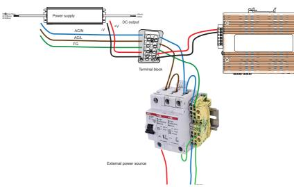
The surge protector becomes worn out after surges. When the indictor widnow changes color, replace the protecor. You can connect wires from its alarm terminal to a camera's DI pins so that you can receive notifications when the protector becomes worn out. Check the surge protector especially after lightning strikes. You can revceive the related alarm by configuring an event via Email, FTP, etc. via the
