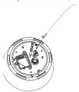
Connect the ground wire to the copper screw hole on the cabinet door.
