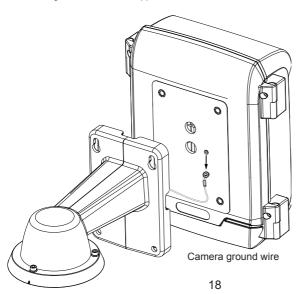
Connect all ground wires (including those from the surge protectors) to one position on the cabinet door, to the terminal block, and then to the external ground.
