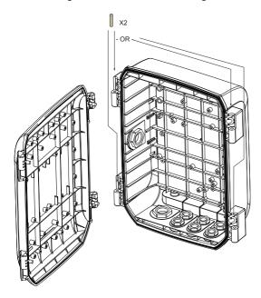
Pass the Ethernet and I/O combo cables through the M20 cable glands, and into the cabinet. You may need to open the cabinet. Secure the camera mount bracket (here a speed dome bracket is shown) to the cabinet. You can then install the camera. Refer the camera's documentation for formation.
