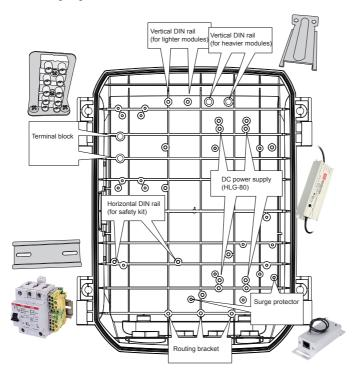
The combination and the choice of components within the cabinet depends on the cameras you want to deploy using this cabinet. Select your devices with the consideration of power consumption, cabling distance, the number of cameras, the operating temperature, and so on. Multiple devices can be stacked as along as the space within the cabinet allows.
