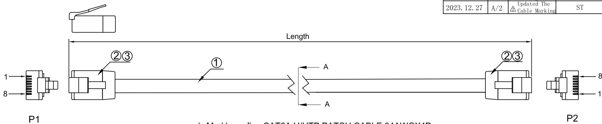
⚠ Marking:roline CAT6A U/UTP PATCH CABLE 34AWGX4P
