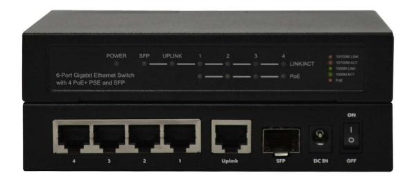
Note: Please turn off the power switch when inserting the DC plug.
