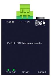
Power over Ethernet provides a way for Ethernet network devices to be powered by UTP cables, including Cat.5, 5e, and 6 rather than by separate power cords. The device is a mid-span injector that can deliver output power supporting proprietary PoE++ 90W Type 4 PDs, 802.3at Type 2 high-power PDs, and 802.3af Type 1 PDs. The injector supports both Fast Ethernet connection and Gigabit Ethernet connection.
