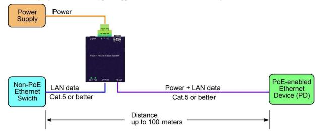
The cable distance including the segment from the injector to the Ethernet device and the segment to PD is no more than 100 meters.
