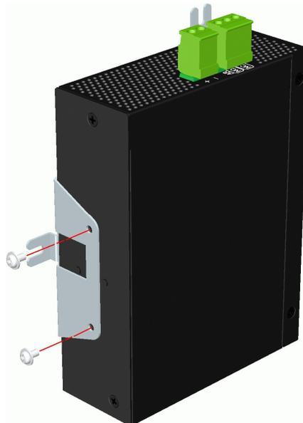
3. Screw the switch unit on a panel. The locations for screws are shown below:
