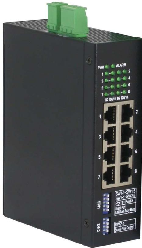
This switch provides eight 10/100/1000Mbps copper ports for the connection of Ethernet, Fast Ethernet, or Gigabit Ethernet devices. With the auto-negotiation function, the switch can detect and configure the connection speed and duplex automatically. The switch also provides auto MDI/MDI-X function, which can detect the connected cable and switch the transmission wire pair and receiving pair automatically. This auto-crossover function can simplify the type of network cables used.
