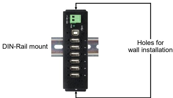
2. Connect the USB cable to the USB-B port on the hub.
