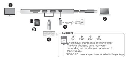
1. Connect a USB-C PD power adapter or a USB-C peripheral device to the unit's USB-C DC-in port, respectively for power redundancy or peripheral device operation.
