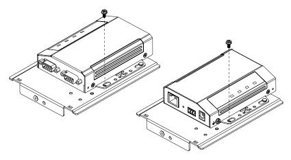
3. Position and align the holes on the VE-RMK1U frame with that of the rack, and secure the frame onto the rack with 2 self-supplied screws, as illustrated below.
