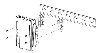
2. Hang the unit onto the DIN rail.
