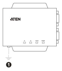
**Note:** Do not omit this step. Proper grounding helps prevent damage to the unit from power surges and static electricity.
