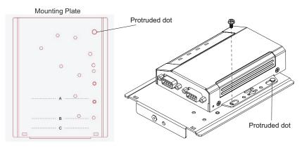
2. Secure the device to the mounting plate using the hexagon head screw supplied. Users can secure the Secure Device Server either with its serial port(s) facing inward or outward.
