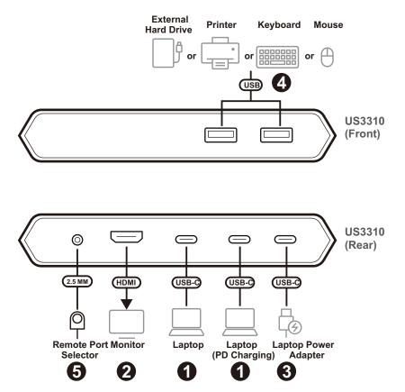
1. Plug the USB-C cable between your computer and/or mobile device into the back of the US3310.
