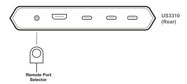
2. Connect one end of the USB Type-C cable to the computer and the other end to the US3310 USB 3.2 Gen 1 Type-C Port 1.
