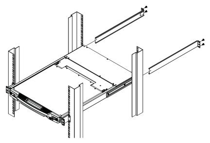
4. After the L-shaped brackets are secured, tighten all the screws.
