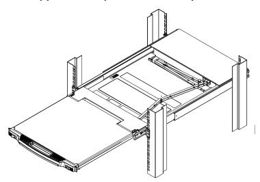
3. Rotate the top panel all the way back to expose the LCD screen.
