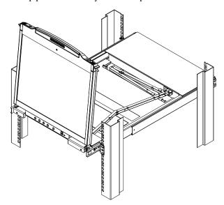
4. Reach underneath and pull the keyboard module all the way out until it clicks into place.
