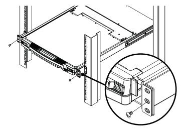
3. While the first person still holds the unit in place, the second person slides the left & right L-shaped brackets into the unit's side mounting brackets from the rear, installing four screws in the brackets to secure them in place.
