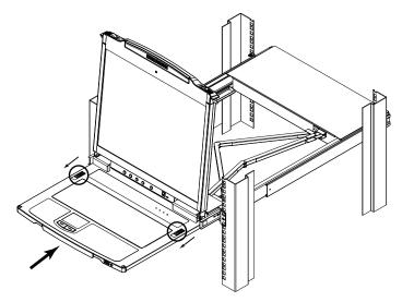
2. Let go of the catches. Using the front handle, push the keyboard module all the way in.
