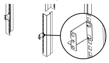
**Note:** Rack screws are not provided to mount the unit. We recommend that you use M5 x P0.8 screws.
