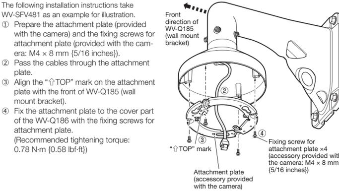
\* The upper right illustration is provided as an example of attaching the attachment plate for a camera model having three attachment mounting screws.
