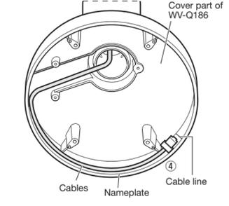
④ After fixing the WV-Q186 on the WV-Q185, lay the cables as shown in the upper right illustration and confirm that the ends of the cables reach the cable line inside the cover of the WV-Q186.
