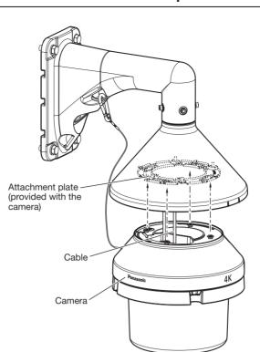
① After connecting the cables to the camera, align the left "|" mark (meaning "OPEN" position) at the 4K mark of the camera. Then, insert the attachment mounting screws (4 points) at the bottom of the camera into the holes of the attachment plate (provided with the camera). After that, align the right "I" mark (meaning "LOCK" position) at the 4K mark of the camera by rotating the camera body clockwise by approx. 15° to fix temporarily.
