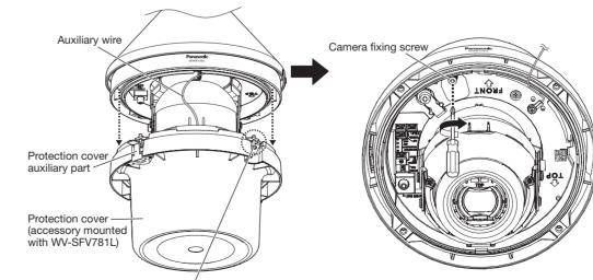
Dome fixing screw (2 pcs.) (The second screw is placed at the opposing side of this screw.)
