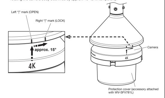
\* The direction of the camera when it is installed on the attachment plate vary by camera. For further information on the installation of a camera, refer to the Installation Guide of the camera to be installed. (The illustration below shows the example for WV-X8570N and WV-S8530N)
