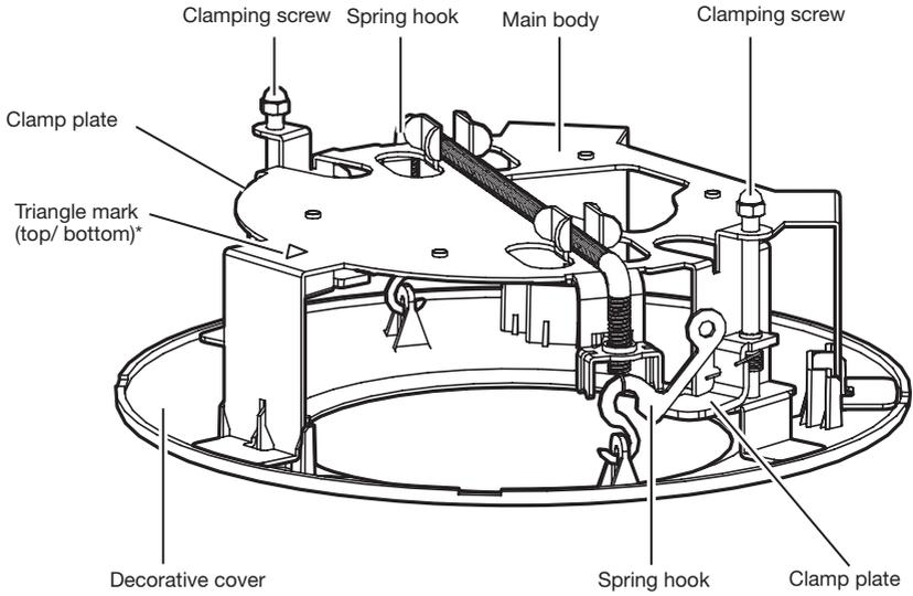
\* Because the triangle mark is engraved on the bracket, it can be seen from both the top and bottom sides.
