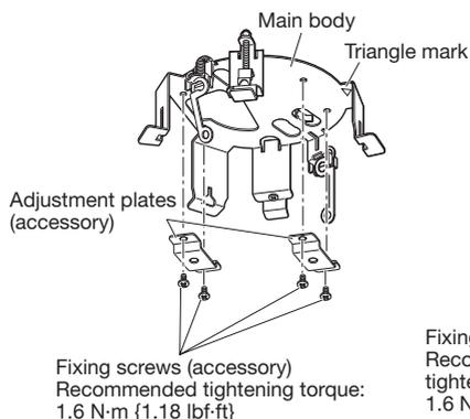
**<When securing the camera body using the attachment plate>**
