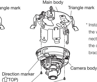
\* Install the camera so that the wiring should be connected from the side of the ceiling mount bracket.
