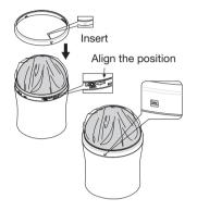
4 Install the camera and remove the protective sheet. See the camera installation guide for further information.
