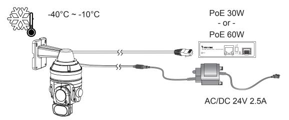
However, when power outage occurs on the DC input, the camera turns to PoE for power supply. In this case, the PoE can only provide 30W or 60W output. The PoE PSE can not deliver sufficient power to drive the onboard heater, and will enter a continuous reset state.
