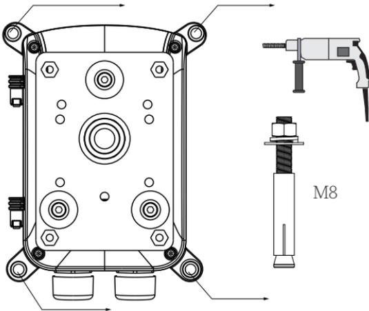
Use the following mounting positions for the camera housings (via AM-21D and AM-21E).
