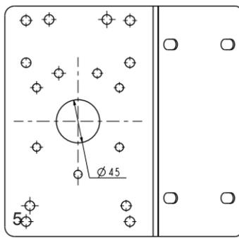
If the power box is directly mounted to wall, drill holes in a diameter of 9.5mm or 3/8", and 4cm deep.
