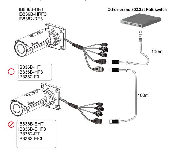
The IB "E" series (heater models) can not be applied in the cascade configuration due to its extra power consumption.
