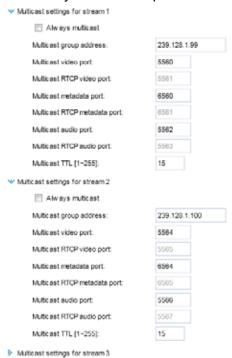
Unicast video transmission delivers a stream through point-to-point transmission; multicast, on the other hand, sends a stream to the multicast group address and allows multiple clients to acquire the stream at the same time by requesting a copy from the multicast group address. Therefore, enabling multicast can effectively save Internet bandwith.
