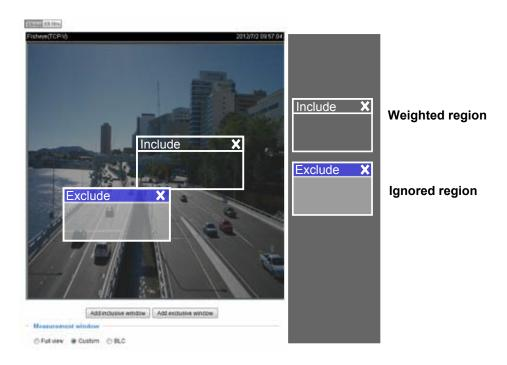
■ BLC (Back Light Compensation): This option will automatically add a "weighted region" in the middle of the window and give the necessary light compensation.
