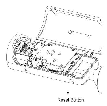
The reset button is used to reset the system or restore the factory default settings. Sometimes resetting the system can return the camera to normal operation. If the system problems remain after reset, restore the factory settings and install again.
