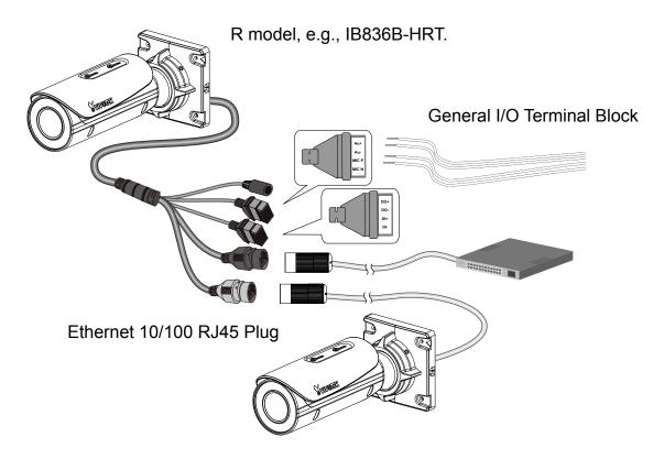
The second LAN port (PoE out, yellow) is available on the IB836B-HRT, IB836B-HRF3, and IB8382-RF3. The R models come without the DC connector.
