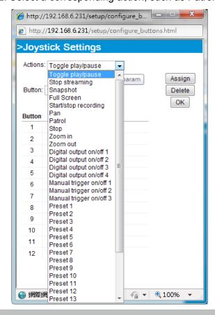
Click the **Assign** button to assign an action to the button. You can delete an association by selecting a button number, and then click the **Delete** button.
