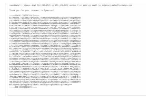
7. Open a new edit, paste the certificate contents, and press ENTER at the end of the contents to add an empty line.
