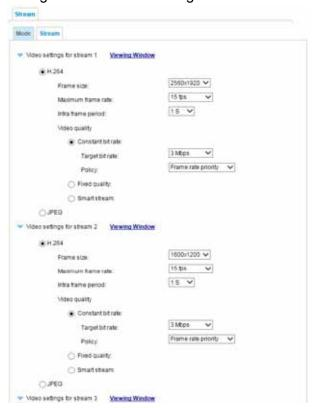
This Network Camera offers real-time H.264 and MJPEG compression standards (Dual Codec) for real-time viewing. If the H.264 mode is selected, the video is streamed via RTSP protocol. There are several parameters through which you can adjust the video performance:
