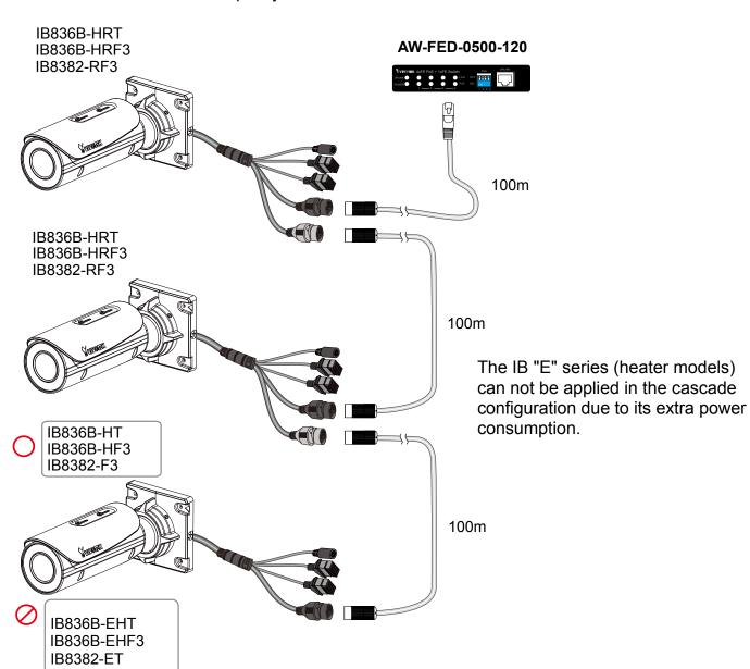
When using an ordinary 802.3at PoE switch (30W output per port), up to 1 IB836B-HRT and 1 IB836B-HT can be cascaded in a configuration with a cabling distance of up to 200 meters.
