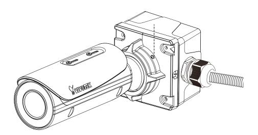
9. Loosen the fastening ring on the mount bracket using a hex wrench, and aim the camera at the area of your interest. When done, tighten the fastening ring.
