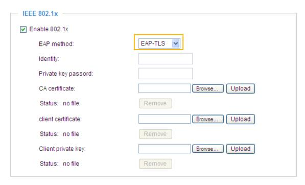
3. When all settings are complete, move the Network Camera to the protected LAN by connecting it to an 802.1x enabled switch. The devices will then start the authentication automatically.
