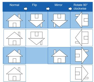
The camera may be installed on a vertical, side-facing, or tilted surface in order to accommodate the interior or exterior design of a building. The interior of a building can be shaped as a narrow rectangular space, such as a corridor. The conventional HD image, such as that of a 16:9 aspect ratio, will be incongruous with its wide horizontal view. With video rotation, the camera can more readily cover the field of view on a tall and narrow scene.
