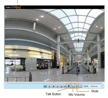
Click to enable audio transmission to the Network Camera; click to adjust the volume of microphone; click to turn off the audio. To stop talking, click again.
