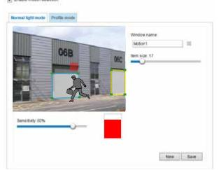
The Percentage Indicator will rise or fall depending on the variation between sequential images. When motions are detected by the Network Camera and are considered to exceed the preset threshold, the red bar rises. Meanwhile, the motion detection window will be outlined in red.
