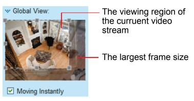
Note that the PTZ buttons on the panel are not operational unless you are showing only a portion of the full image. If the live view window is displaying the full view, the PTZ buttons are not functional.
