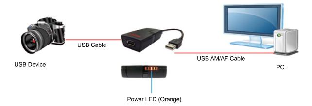
The USB Isolator unit is installed in-line between the PC and a connected USB device.
